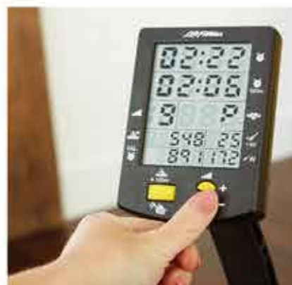
Console Displays: Time, Distance, Strokes/Minute, 500-Meter Split Time, Calories/Hour, Watts
